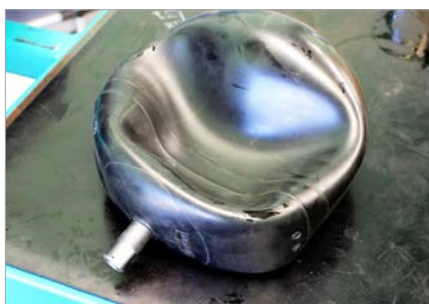
12. Inspect the bladder. In cases where there are signs of damage, wear or swelling then the bladder should be replaced. Refer to page 74 and 75 outlining potential damages, causes and response.
