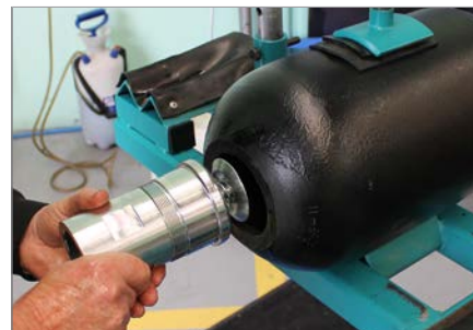
10c. The fluid port can then be removed from the shell.
