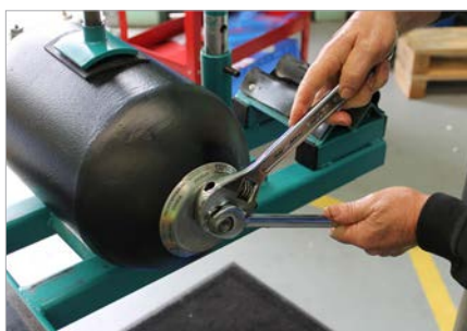
14. Tighten locknut to the bladder stem. Ensure that when tightened the bladder stem does not rotate.
