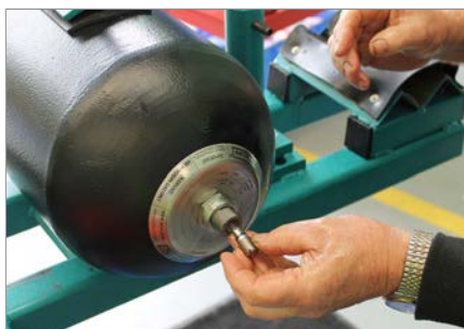
5. Remove the gas valve assembly or gas valve core.
