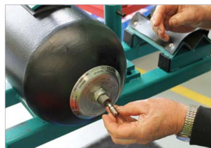
15. Fit the gas valve assembly.
