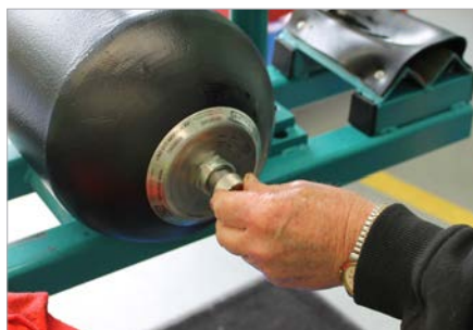
16. Fit the gas valve assembly cap.
