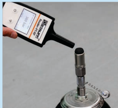
Connected through SSK test coupling
