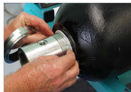
9. Remove the nylon back-up washer along with the O-Ring.
