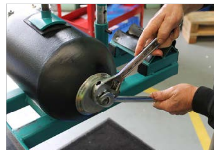
6. Remove the bladder locknut and nameplate.
