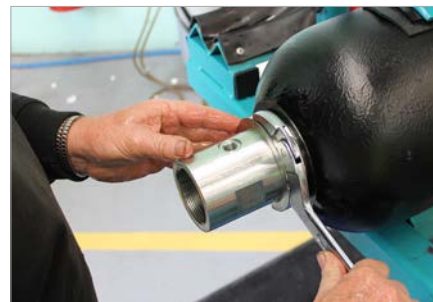
12. Attach first the flanged washer and then the locknut. Ensure the locknut is tightened using an appropriate spanner.
