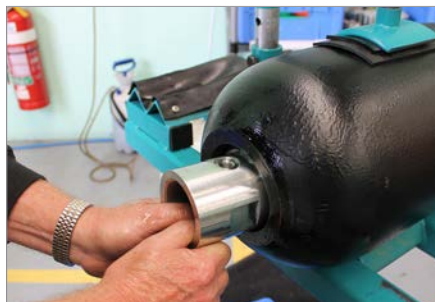
10a. Remove the fluid port assembly by first pushing the fluid port back into the inside of the shell.
