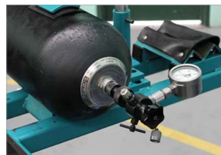
3. Attach STAUFF pre-charging head and release any pre-charge from the accumulator.
