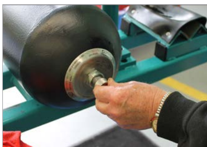
2. Remove the gas valve assembly cap.
