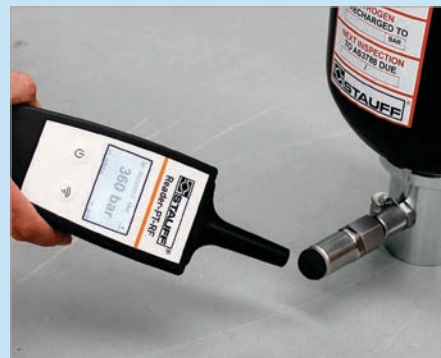
Connected through fluid port
